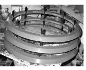
On a standard Dalek, the neck section is almost always made from wood — either MDF or plywood — as is the inner part of the neck, (the neck bin) which holds the
