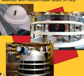
them stay in place when outside. The eyestalk and gun were lit by fully insulated twelve volt light-emitting diodes, with the wires positioned in order to stop any rainwater that got to them from trickling down and earthing out the circuits. To finish it off, the parts were sprayed with weather-proof exterior paint.
